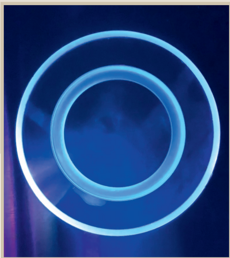
Figure 4. Cleaning agent residues made visible on a component. In high-purity cleaning, the necessary cleaning chemistry is often a major challenge in achieving high cleanliness requirements
